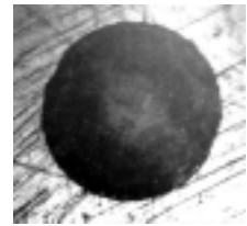
Scratches due to incomplete polishing
